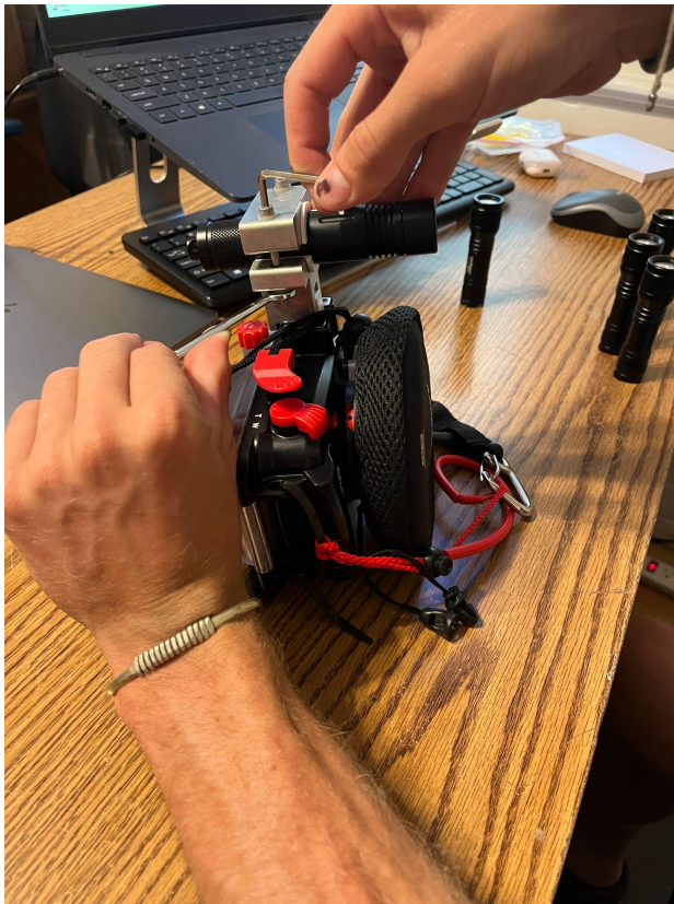
Figure 4. Clockwise from Left, A) tools needed for mount repair require a 3mm allen wrench, and either a 7mm wrench or some other tool (e.g.) pliers to grip the bottom nut to hold still while tightening/loosening the bolt
