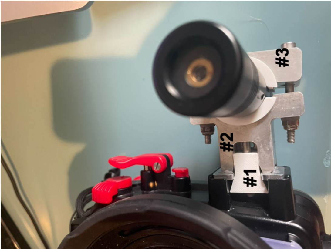
Figure 2. Close up of the laser and mount. #1 is the flange that attaches the metal mount to the camera housing - this piece is made of plastic and will be the most likely source of breakage, if any. #2 is the lower mount. #3 is the upper mount.
