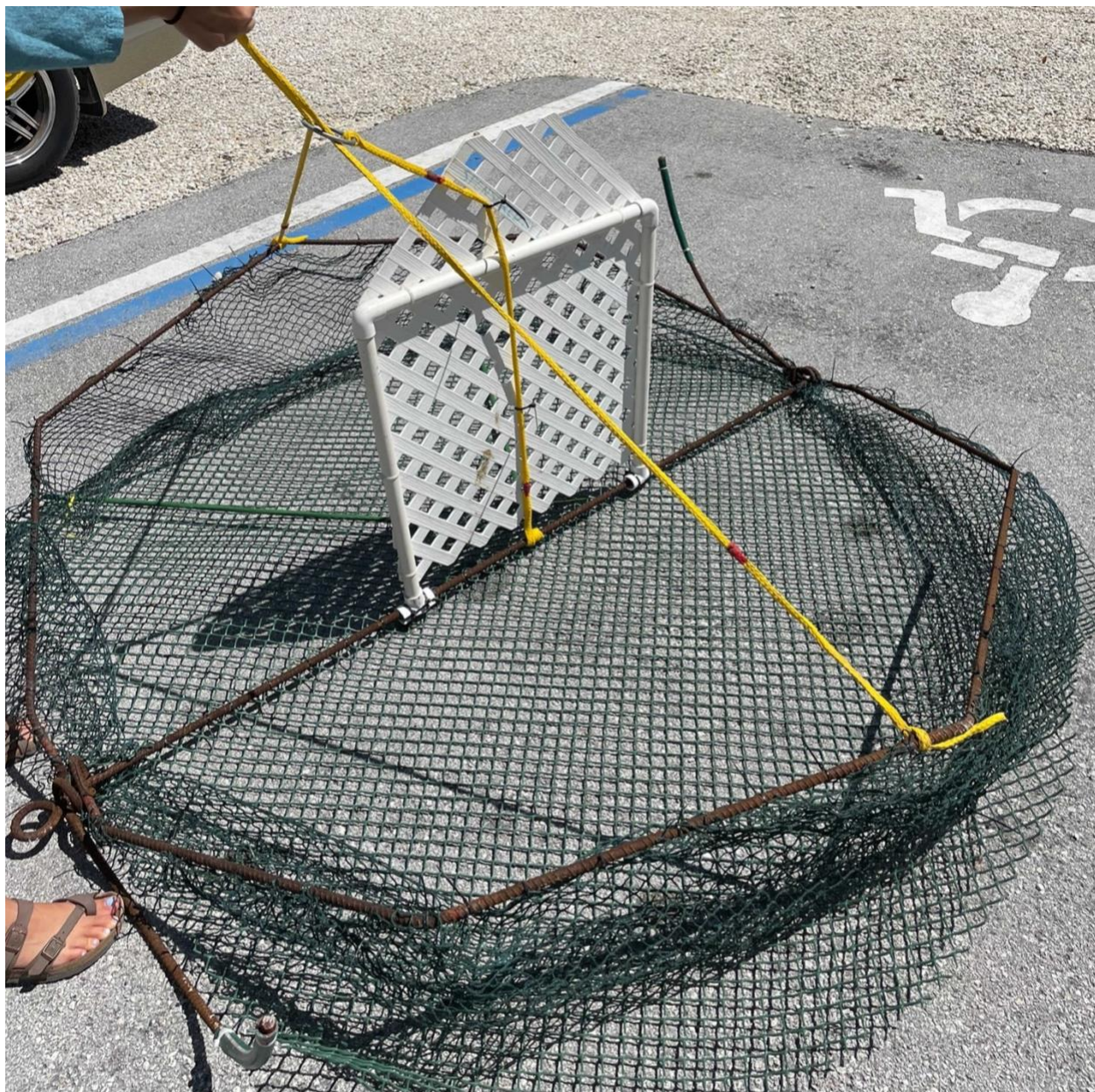
Figure 10. Design 8, “Baffle Design” about 12 inches of netting is attached to rigid plastic mesh, creating an accordion-like design.
